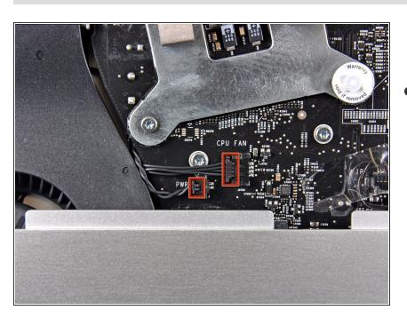
Disconnect the CPU fan and power button by pulling their connectors toward the left edge of the iMac.
