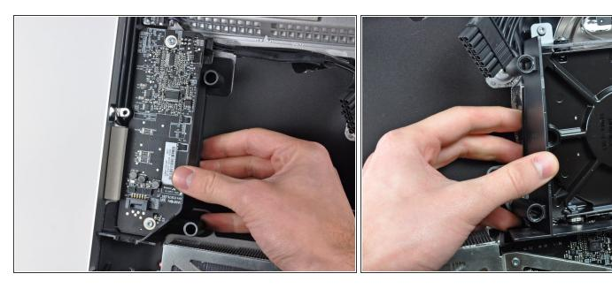
Remove the plastic ducts from the side of the LED driver board and the hard drive by pulling them away from the outer case.
