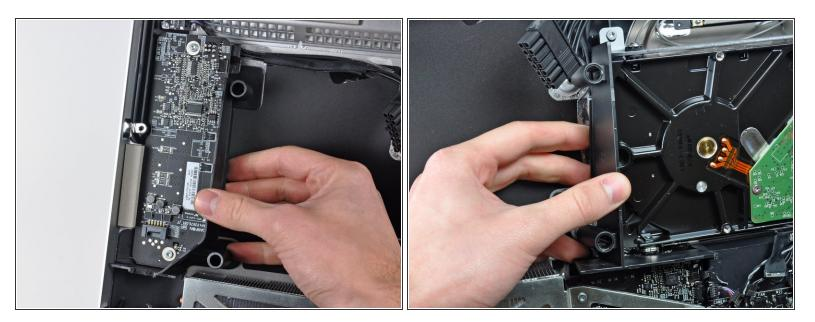
• Remove the plastic ducts from the side of the LED driver board and the hard drive by pulling them away from the outer case.
