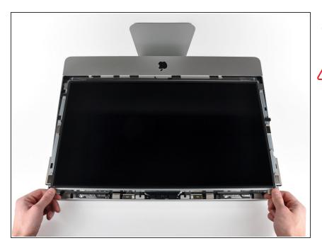
• Slightly lift the top edge of the display out of the outer case.
