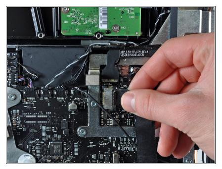
Disconnect the audio port cable by pulling its connector toward the right side of the iMac.
