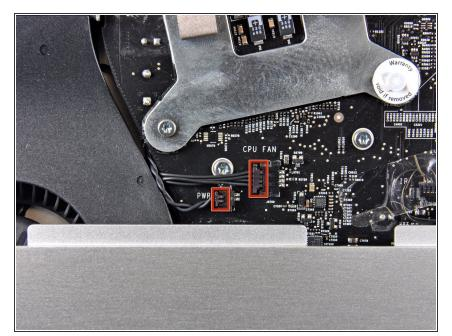
Disconnect the CPU fan and power button by pulling their connectors toward the left edge of the iMac.
