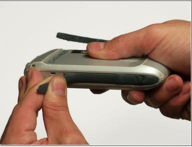
• The bumpers on the top and bottom of the phone can be removed by simply "peeling" them off.
