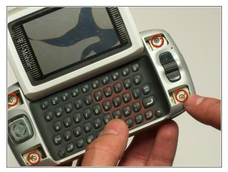
Use the T6 Torx Screwdriver to remove the 4 screws that are underneath the 4 buttons you removed in step one.
