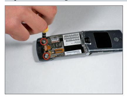
Unscrew the two screws holding the plastic speaker cover to the phone with a T5 screwdriver
