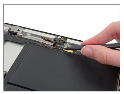
Using the tip of the spudger, flip up the retaining flap on the microphone cable ZIF connector.
