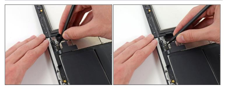
• Flip up the retaining flap on the home button ribbon cable ZIF connector.
