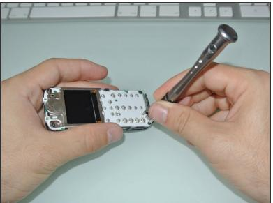
Remove the 4 T6 Torx screws
