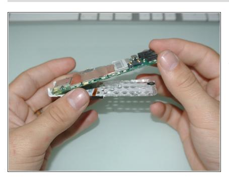
The last thing you need to doto access the Logic Board is to separate the Keyboard/Screen block just taking apart with your fingers.
