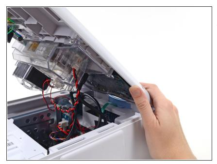
*i* Support the rear housing while you disconnect the cables in the following steps.
