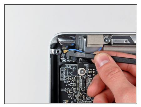
Use the flat end of a spudger to pry the Bluetooth antenna cable connector up off the Bluetooth board.
