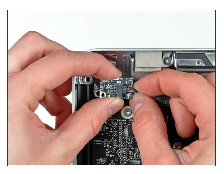
Disconnect the Bluetooth cable by pulling its connector away from the socket on the Bluetooth board.
