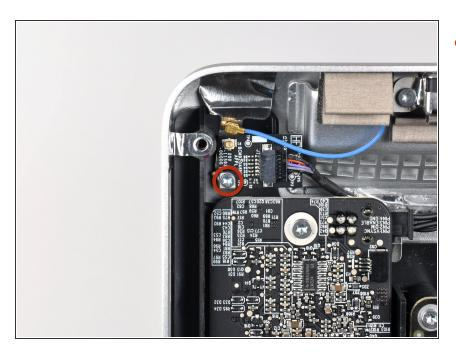
Remove the single 6.6 mm T8 Torx screw securing the Bluetooth board to the outer case.
