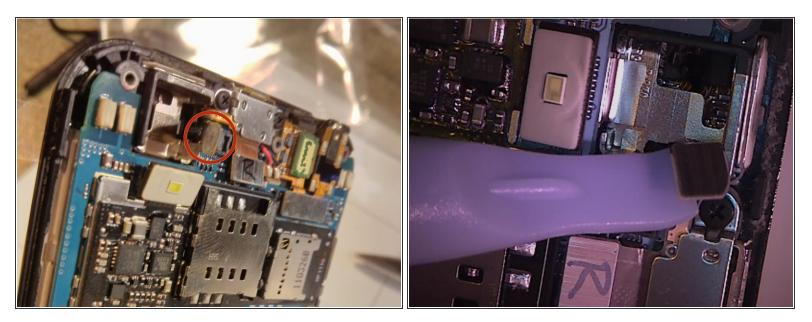
don't forget to remove the little connector of screen, with a tool, right next to the empty slot of the camera.
