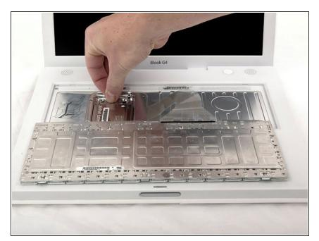
Push the wire clasp away from the AirPort card and toward the display, then rotate up to free it from the RAM shield.
