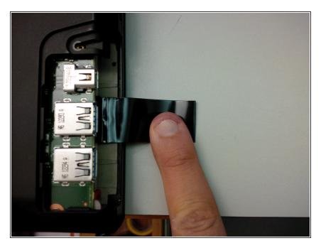
Insert a spudger (or a similar tool) under the loop of the black pull tab, and gently pull it out from above the hard drive.
