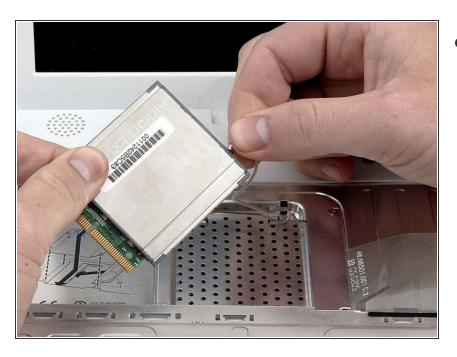
Hold the AirPort card in one hand and use your other hand to remove the antenna cable.
