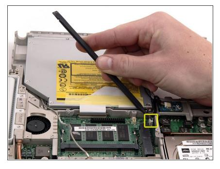
Disconnect the Bluetooth cable from the logic board.
