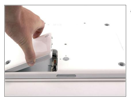
Lift the battery out of the computer.
