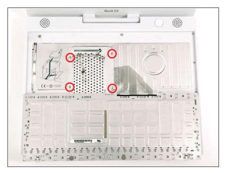
Remove the four silver Phillips screws that secure the RAM shield.
