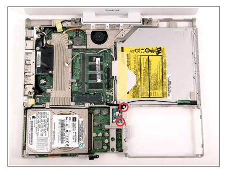
Remove the two Phillips screws securing the Bluetooth assembly to the metal framework.
