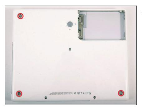
Remove the three newly-revealed Phillips screws.
