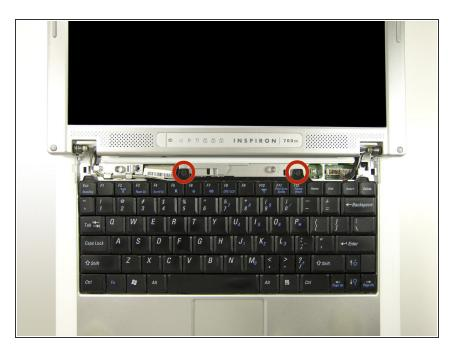
Remove the two Phillips screws securing the keyboard.
