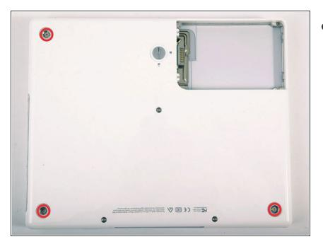
Remove the three newly-revealed Phillips screws.
