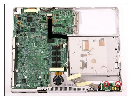
Remove the two Phillips screws securing the DC-In board.
