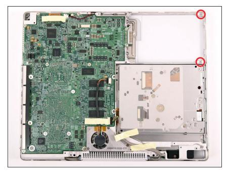
Remove the two Phillips screws from the battery compartment.
