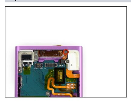
Remove the 1.4 mm Phillips #000 screw from the antenna cable.
