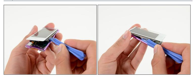
Continue prying along the edges under the front panel assembly, releasing the clips and adhesive along the sides of the device.
