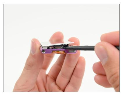
Use a spudger to press the midframe screw tab up and out of the rear case.
