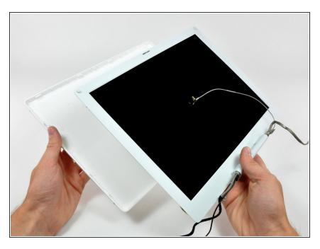
Lift the rear bezel off the display.
