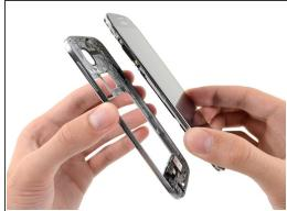
Remove the midframe from the display assembly.
