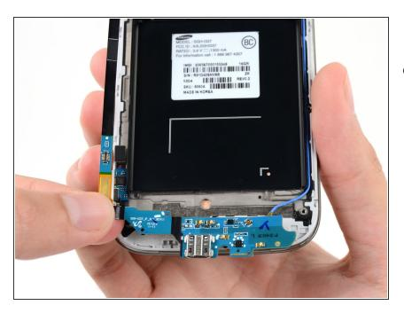
Remove the USB board from the display assembly. To reassemble your device, follow these instructions in reverse order.
