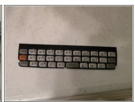
• The keypad cover is easily replacable, and simply lifts out.
