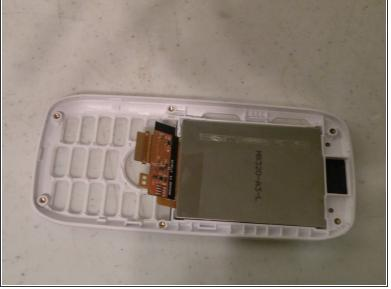
Unfortionatly, the LCD panel is held in place by a heavy adhesive, and removal will almost certianly crack the screen, so only remove it if you are replacing the screen.
