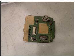
Now, to remove the board, use a flathead screwdriver or spudger to clear the tab on one side, then remove the board completly, similarly to the logic board.
