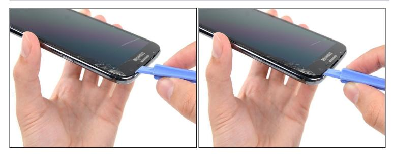
• Push the plastic opening tool down to free the corner of the midframe from the display assembly.
