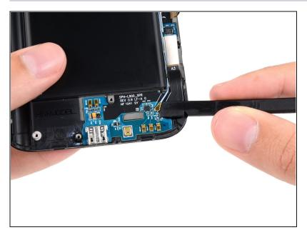
Use the flat end of a spudger to disconnect the antenna cable connector from the USB board.
