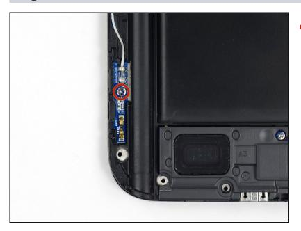
Remove the 3 mm Phillips #00 screw securing the antenna board to the display assembly.
