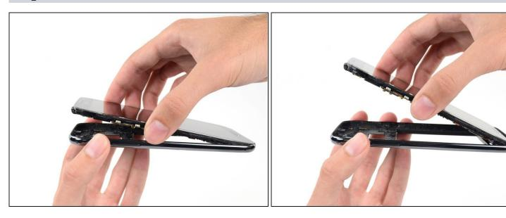
• Lift the display assembly out of the midframe.
