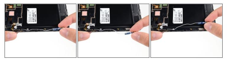
Gently de-route the antenna cable from its channel in the display assembly.
