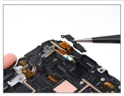
• Remove the front-facing camera bracket.
