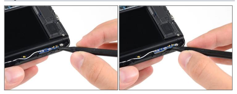
• Insert the tip of a spudger under the antenna board to free it from the adhesive holding it to the display assembly.
