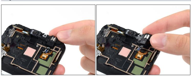
Grasp the headphone jack portion of the assembly and lift it out of its groove in the display assembly.
