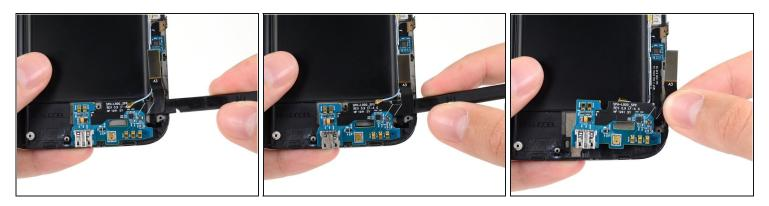
• Push the flat end of a spudger under the USB board to separate it from the display assembly.
