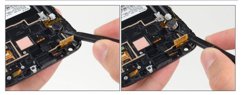
Insert the tip of a spudger under the vibrator to free it from the adhesive holding it to the display assembly.
