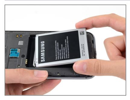
• Remove the battery from the midframe.
