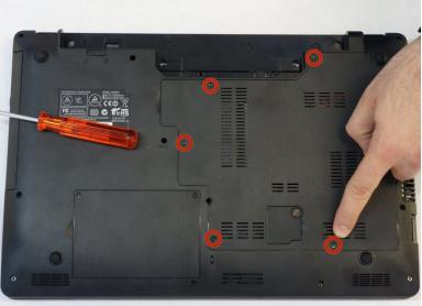
Using a Philips #1 screwdriver, unscrew the 5 screws securing the cover.
