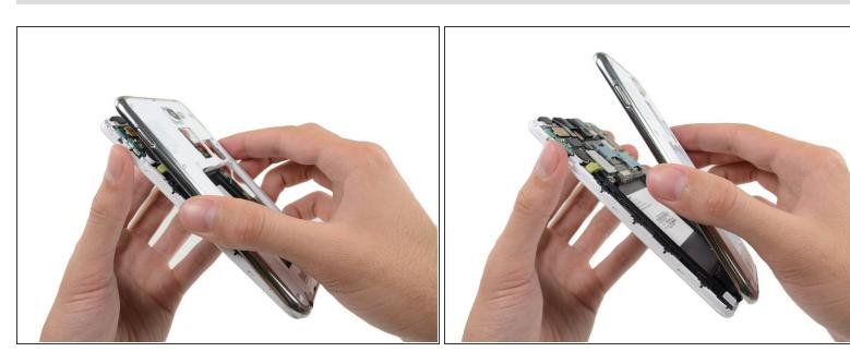
Remove the midframe from the display assembly.
