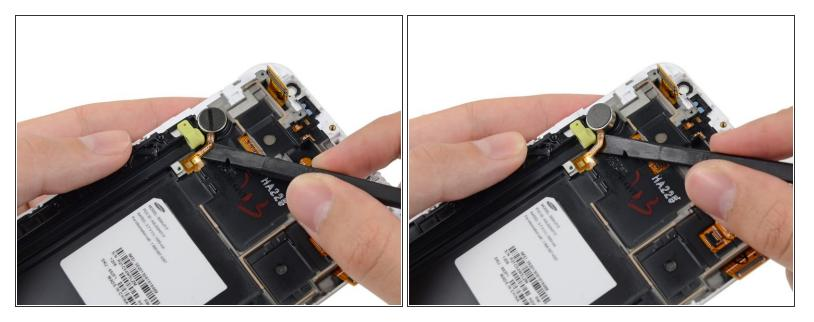
• Insert the flat end of a spudger under the vibrator connector cable, and pry it up from the adhesive.
