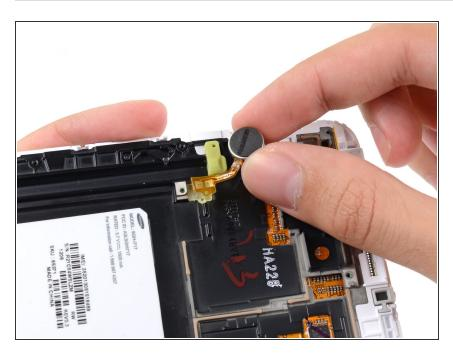
Remove the vibrator from the display assembly.
