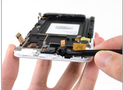
Use the tip of a spudger to pry the headphone jack/earpiece speaker assembly out of its recess in the display assembly.
