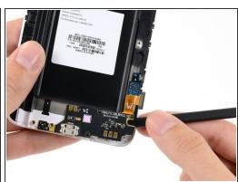
Push the flat end of a spudger under the USB board to separate it from the display assembly.
