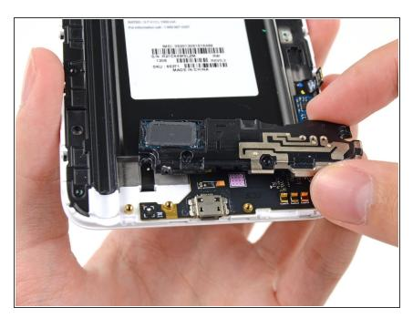
Lift the speaker enclosure from the display assembly.
