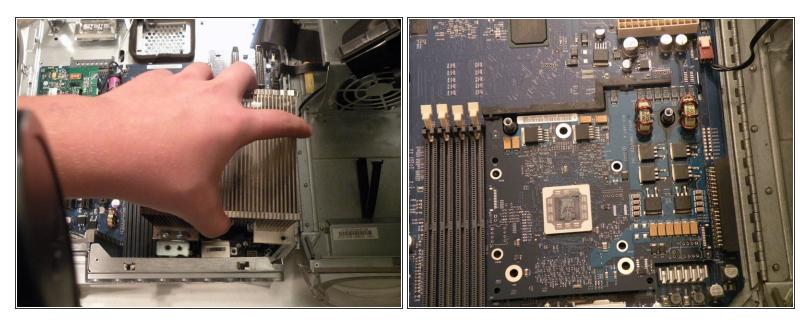
• Now, lift the heatsink up off the computer, it is pretty heavy, because it's a giant block of aluminum.
