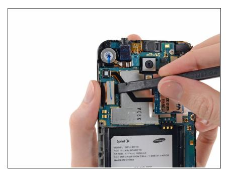
Use a spudger to disconnect the display cable connector.
