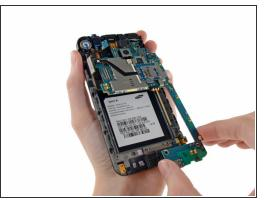
• Lift the micro-USB end of the motherboard away from the display assembly and pull it down.
