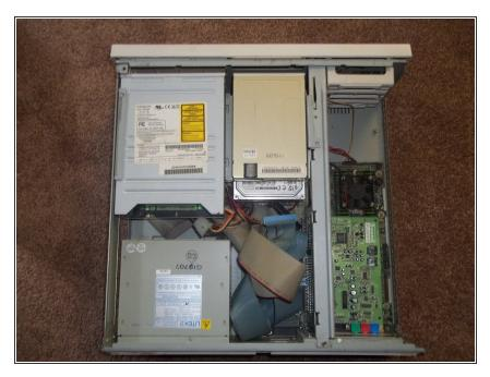
Slide the drive cage back. An easy way to do this is the push on the optical drive from the front.
