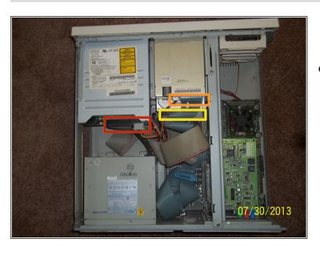
Once the screws are removed, disconnect all cables from the optical drive, hard drive and floppy drive.
