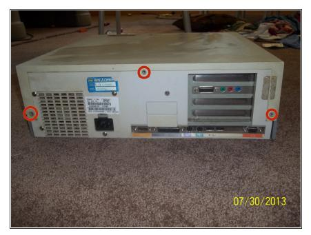
Using a Phillips screwdriver, remove the three Phillips head screws (circled in red) from the back of the computer.
