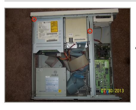
Remove the two Philips head screws with your Philips screwdriver. You may have to
