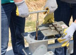
Remove the rod vise from the tank.
