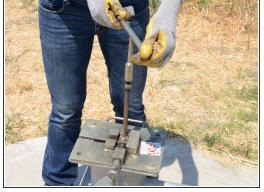
Screw a T-handle onto the top of the pump rod. Tighten the T-handle up against the jam nut.
