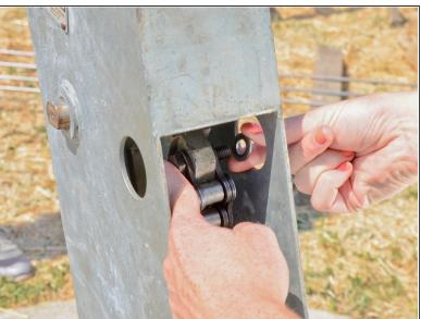
Remove the washer from the chain bolt.
