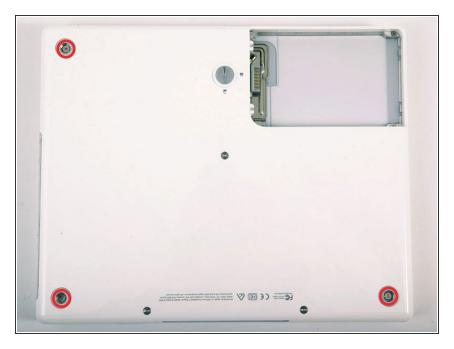
• Remove the three newly-revealed Phillips screws.
