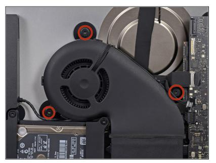
Remove the three 12.3 mm T10 shoulder screws from the fan enclosure.
