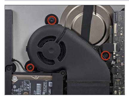
• Remove the three 12.3 mm T10 shoulder screws from the fan enclosure.
