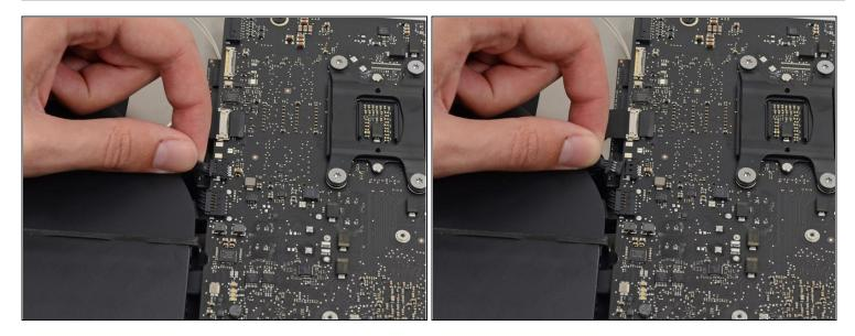
• Disconnect the fan cable connector from its socket on the logic board.
