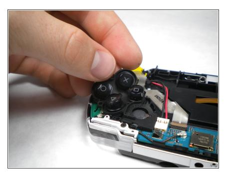
After removing the LCD Screen, the Button Pad should be easy to remove.
