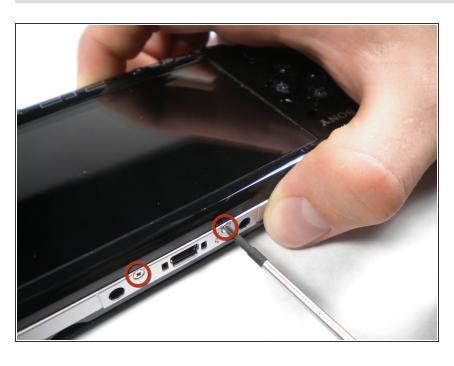
Next, unscrew the two screws located at the top of the PSP.
