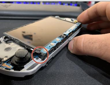
Push the homebar to the right to release the tab located on the right side of the LCD screen.
