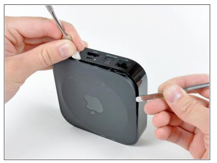
As the device base is firmly clipped, insert two metal spudgers to gently release the first clips.
