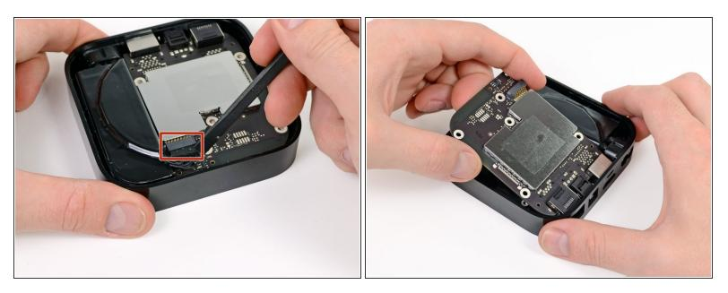
Disconnect the power supply connector from the logic board with a spudger.
