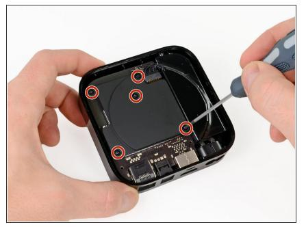
Use a philips screwdriver to remove the 5 screws securing the metal heat sink. On Rev A (A1469) you need a T7 srewdriver
