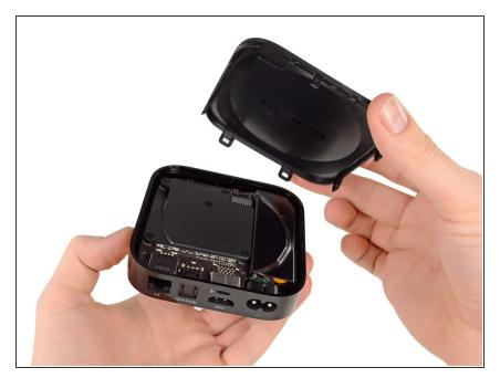
• Continue releasing the last plastic clips with your hands taking care not to break any of the plastic elements attached to the base.
