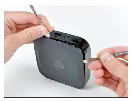
As the device base is firmly clipped, insert two metal spudgers to gently release the first clips.
