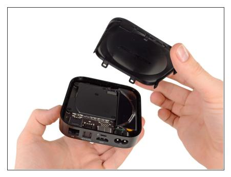
Continue releasing the last plastic clips with your hands taking care not to break any of the plastic elements attached to the base.
