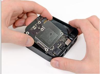
Disconnect the power supply connector from the logic board with a spudger.
