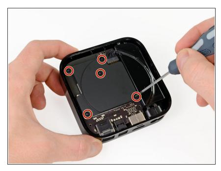
Use a philips screwdriver to remove the 5 screws securing the metal heat sink. On Rev A (A1469) you need a T7 srewdriver
