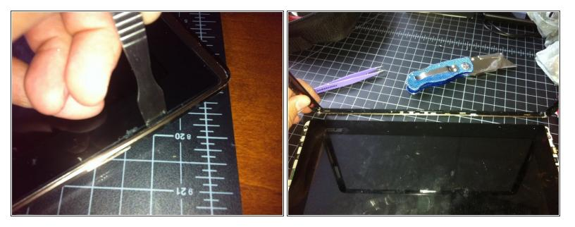
• I used a metal opening tool to spearate the bezel from the front of the unit. Once I had it separated in one area it was relatively easy to spread it using my fingertip. I then worked around the bezel until it popped off.
