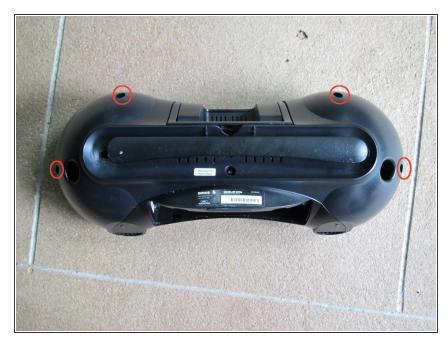
Begin by unscrewing the four recessed screws in the rear of the boombox. They don't seem to be magnetic, and they may not pop out immediately.
