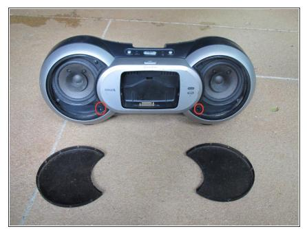
There are screws now accessible near the bottom of each side under the mesh, near the center of the boombox. Once you remove these, the faceplate will come right off.
