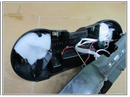
Now you can get to some of the electronic components. Only eight screws separate you from the inside of the boombox. Undo the screws and fix up the inside to your heart's content.
