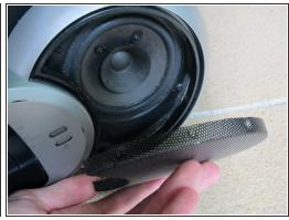
Next, you will need to remove the mesh that covers the speakers. Using the flathead screwdriver, start prying near the top or bottom of the mesh, near the center. The 'corners' come up more easily. Once you have part of the mesh pulled out, go around the outside and use indents in the mesh to pry it out. Try not to bend the mesh very much.
