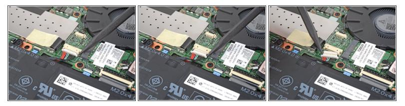
Use the pointed end of a spudger to push each side of the battery connector until it comes out of the socket.
