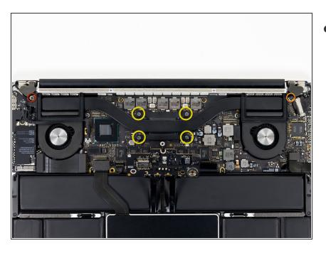
Remove the following screws securing the heat sink to the logic board assembly:
