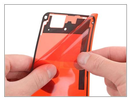
Peel away the plastic lining to expose the frame side of the replacement adhesive.
