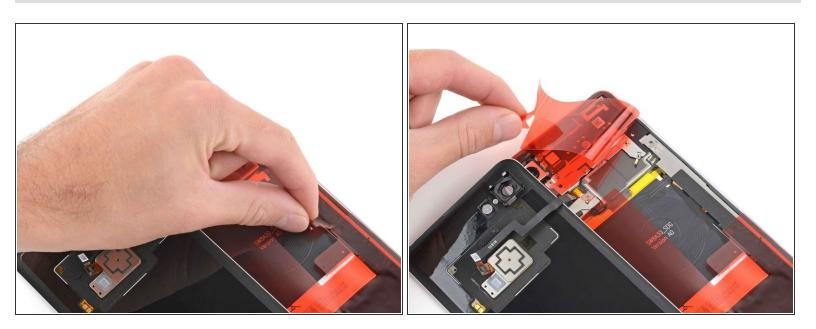
Peel away the plastic lining to expose the back cover side of the adhesive.
