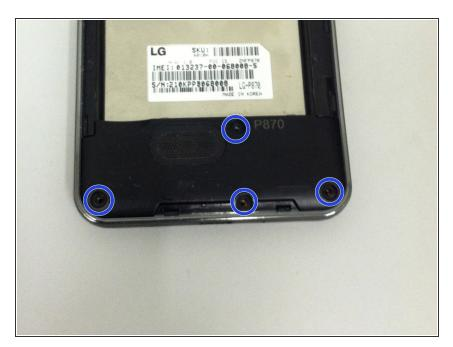
Remove the 4 Phillips 00 screws securing the speaker assembly to the phone housing.
