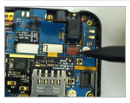
Release the headphone jack's flex cable from its connector
