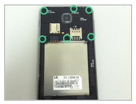
Remove the remaining 6 screws securing the plastic frame to the back housing
