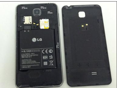
• Turn the device over and pull the back plastic cover off by inserting your fingernail into the opening at the bottom of the phone and gently pulling.
