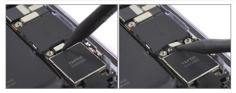
• Use the pointed end of a spudger to disconnect the Taptic Engine by prying the connector straight up from its socket.
