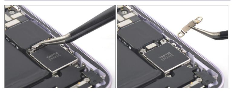
• Use a pair of tweezers to remove the Taptic Engine connector bracket.
