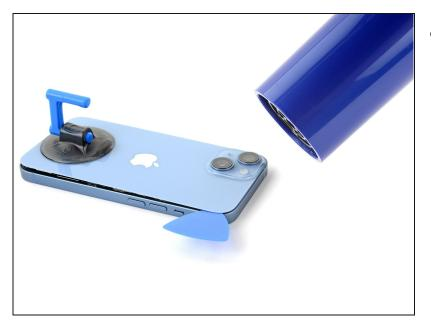
• Use a hair dryer to heat the top edge of the iPhone for 90 seconds or until the rear glass is slightly too hot to touch.
