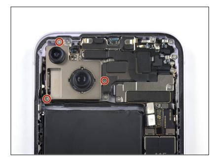
Use a Phillips screwdriver to remove the three 2.1 mm-long screws securing the rear-facing camera assembly.
