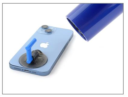
• Use a hair dryer to heat the right edge of the iPhone (the edge with the power button) for 90 seconds or until the rear glass is slightly too hot to touch.
