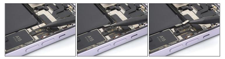
• Use a spudger to disconnect the two rear-facing camera assembly cables by prying the connectors straight up from their sockets.
