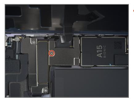
Use a Y000 screwdriver to remove the single 1.0 mm-long screw securing the charging coil connector cover.
