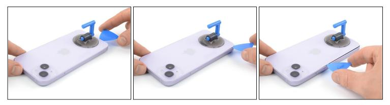
• Slide the opening pick around the lower left corner and up the left edge of the iPhone, slicing through the adhesive holding the rear glass in place.
