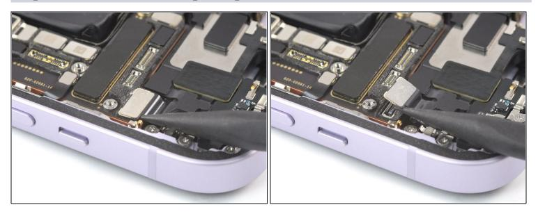
• Use a spudger to disconnect the earpiece cable by prying the connector straight up from its socket.
