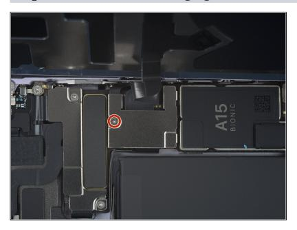
Use a Y000 screwdriver to remove the single 1.0 mm-long screw securing the charging coil connector cover.
