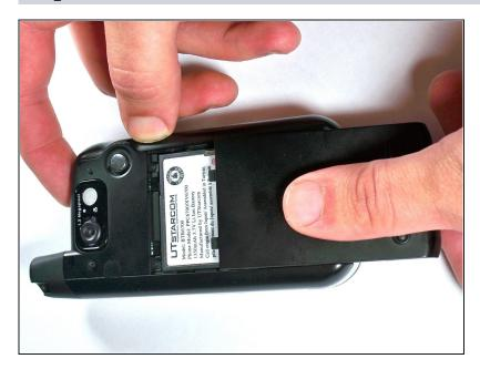
Remove the battery cover by pressing and sliding the cover down and off of the phone.
