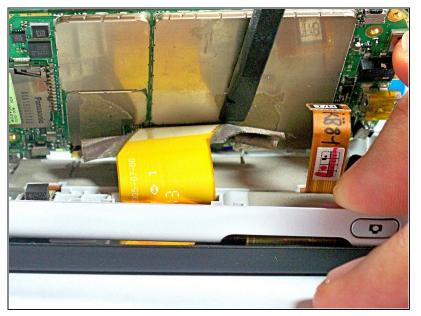
• Use the spudger to peel away the tape from the connector.
