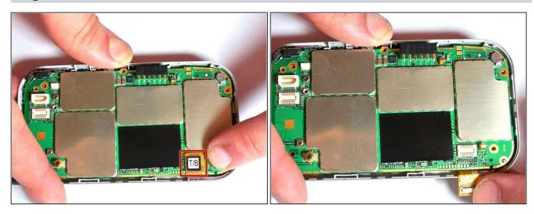
• With your fingers, disconnect the keyboard cable from the motherboard. The cable is orange with the letters T/B printed on the connector.
