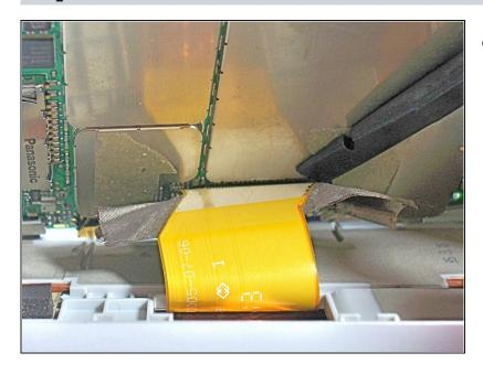
Using the spudger, pry away the display cable connector from the motherboard. The motherboard is now completely disconnected.
