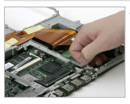
Disconnect the reset button from the logic board. (this part is not present on later models)
