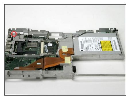
Remove the single Phillips screw that secures the logic board to the metal framework and remove the metal shielding.
