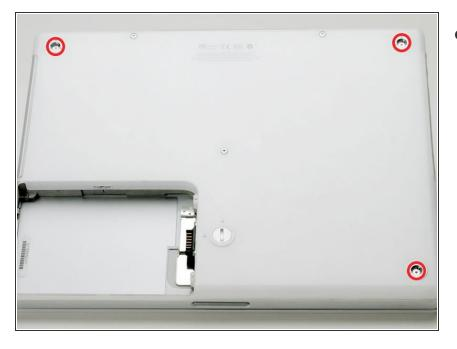
Remove the three newly-revealed Phillips screws.
