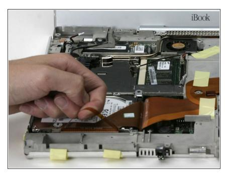
At the front edge of the hard drive, lift up on the transparent orange tape to disconnect the ribbon cable from the main board.
