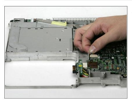
Disconnect the DC cable from the logic board.
