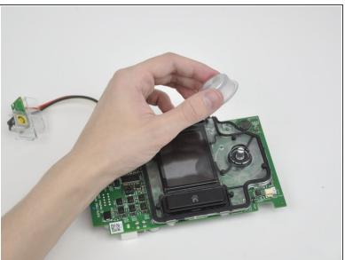
Pry the knob away from the screen cover plate using a spudger or opening tool, while supporting
