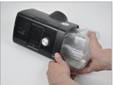
Remove the water tub by gently pulling it out.
