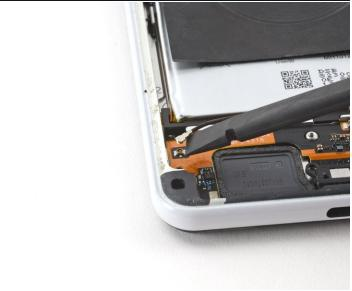
• Use the flat end of a spudger to pry up and disconnect the black coaxial cable connector from the charging assembly.
