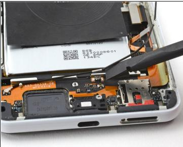
Use the flat end of a spudger to pry up and detach the black coaxial cable from its clip on the charging assembly.
