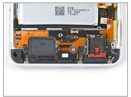
Use a T3 Torx screwdriver to remove the 3.9 mm screw securing the USB-C port bracket to the frame.
