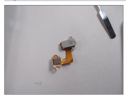
Carefully lift the headphone jack off the removed panel.
