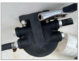
Attach 10 mm socket to a 1/4" ratchet wrench and loosen the bolt on the left side and then the right.
