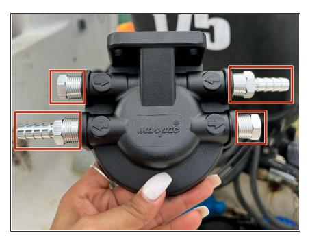
Screw the four bolts with the thread sealant to the new top base of the new fuel filter.
