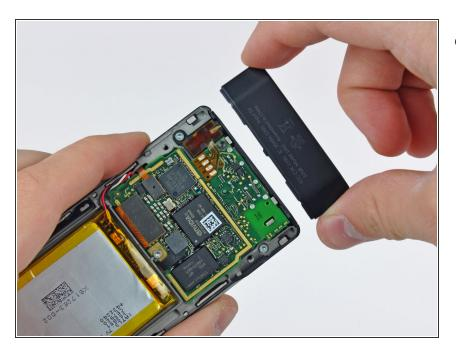
Carefully slide the lower rear panel away from the Zune.
