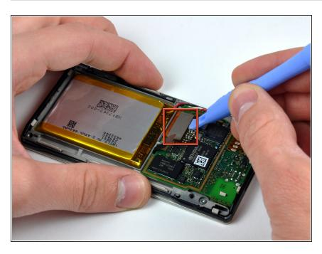
Use a Zune opening tool to pry the OLED display ribbon cable connector up off the logic board.
