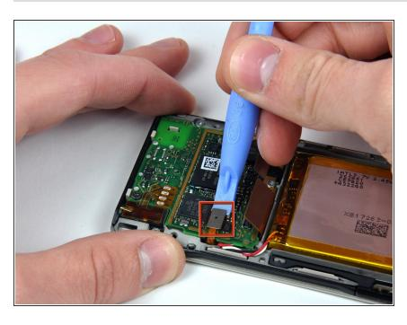
Use a Zune opening tool to pry the control ribbon cable up off the logic board.
