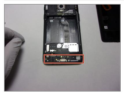
Properly orient the new speaker unit and use a Phillips #000 screwdriver to replace the eight screws removed from the previous step.
